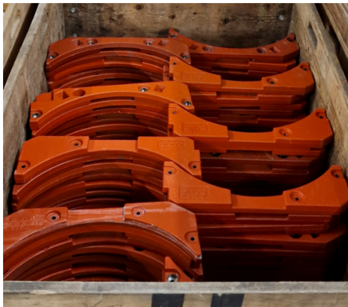
Counterweights made of cast iron – ready for re-use in washing machines
