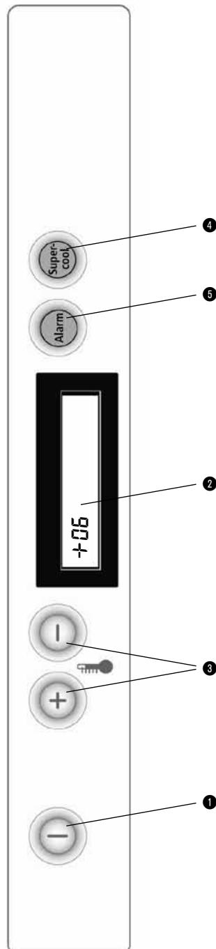
After 10 minutes an alarm sounds; reset by pressing the alarm acknowledgement.
