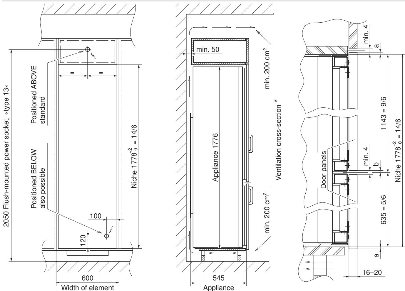
\* Allow a gap – at the top and bottom – less than the width of the appliance to ensure proper ventilation (sheets 5–13 in the technical guide on kitchen planning and design from the Swiss Kitchen Association (KVS)).
