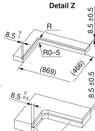
Steel angle bonded or screw mounted
