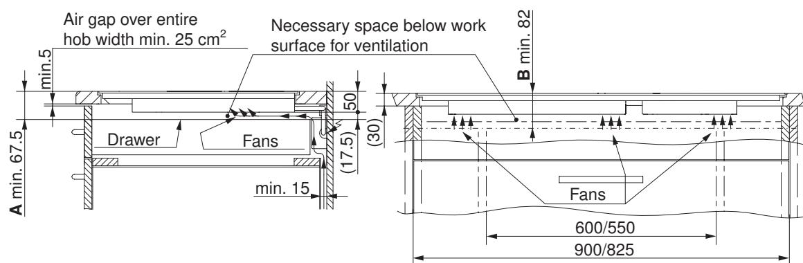
= Necessary space below the work surface for the ventilation of the appliance.
