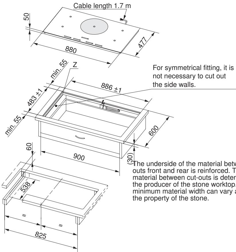
The underside of the material between cut-outs front and rear is reinforced. The width of material between cut-outs is determined by the producer of the stone worktop. The minimum material width can vary according to the property of the stone.
