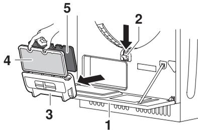
**Cleaning the filter mat in front of the heat pump**
