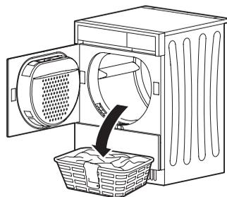
If the appliance door is opened during the «Cool down» phase, the programme is aborted and the indicator lights and display go out.
