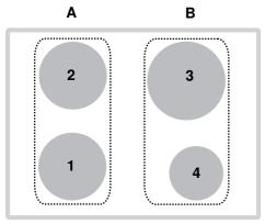
PowerPlus cannot be used with both cooking zones of a group ( $\bf A$  or  $\bf B$ ) at the same time. If PowerPlus is activated with both cooking zones of a group, then the power output is reduced for the cooking zone that was first selected.
