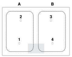
PowerPlus cannot be used with both cooking zones of a group ( $\bf A$  or  $\bf B$ ) at the same time. If PowerPlus is activated with both cooking zones of a group, then the power output is reduced for the cooking zone that was first selected.
