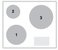
PowerPlus cannot be used at the same time as the cooking zones **1** and **2**. If PowerPlus is activated with both cooking zones, then the power output is reduced for the cooking zone that was first selected.
