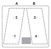
PowerPlus cannot be used with both cooking zones of a group (**A** or **B**) at the same time. If PowerPlus is activated with both cooking zones of a group, then the power output is reduced for the cooking zone that was first selected.
