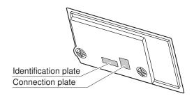
► Affix the second identification plate (supplied) in an accessible position behind the front of the fitted cabinet beneath the appliance.
