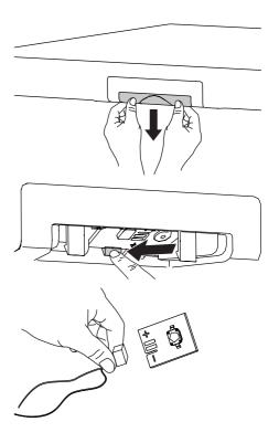
Reverse this procedure to insert the new LED light.
