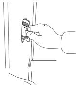
► Disconnect the plug connection 1 for the LED light.
