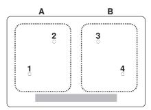
PowerPlus cannot be used with both cooking zones of a group ( $\bf A$  or  $\bf B$ ) at the same time. If PowerPlus is activated with both cooking zones of a group, then the power output is reduced for the cooking zone that was first selected.
