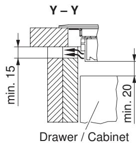
Mounting cut-outs in side walls left/right for a niche width of 900 mm, necessary for the ventilation of the appliance.
