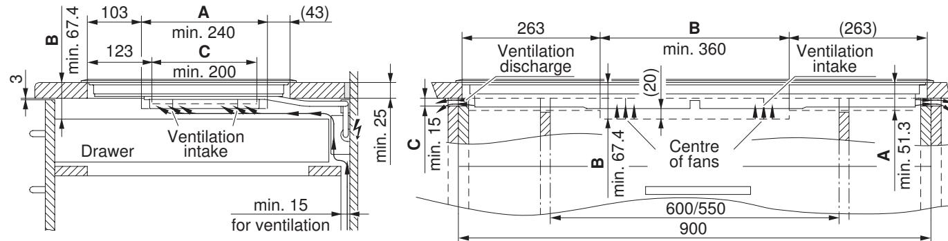
**A** Necessary space below the work surface for the appliance, only for niche width 600/550 mm.
