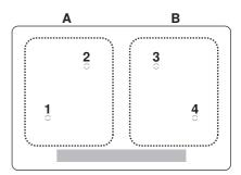
PowerPlus cannot be used with both cooking zones of a group (**A** or **B**) at the same time. If PowerPlus is activated with both cooking zones of a group, then the power output is reduced for the cooking zone that was first selected.
