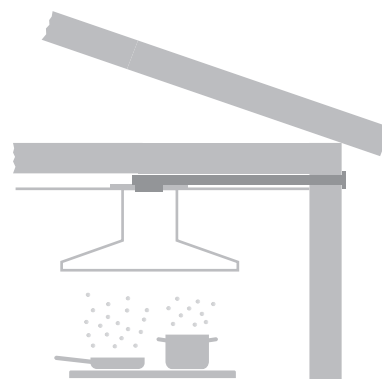
With concealed exhaust duct, e.g. suspended ceiling with flat channel exhaust air conduit
