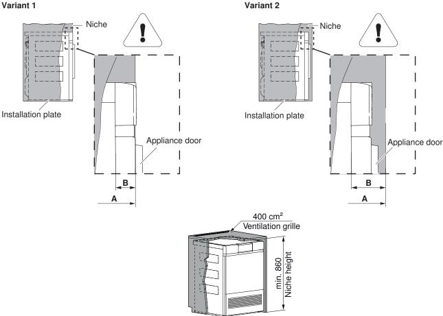
The heat given off from the rear of the appliance must be conducted out of the niche. By means of 2 ventilation grilles P33.002 or a ventilation cut-out of min. 400 cm<sup>2</sup> in the niche cover ensure there is a supply of fresh air via the connection opening.
