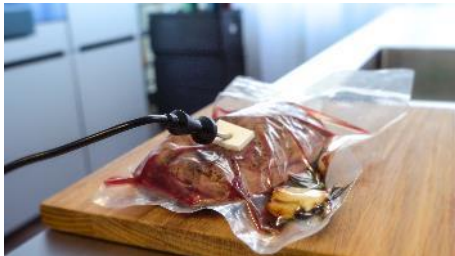
Photo 2 Thanks to the new sealing pads, the food probe temperature of a piece of meat can be monitored even when cooking with Vacuisine.
