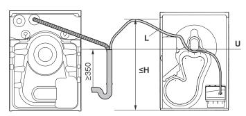
► Position the drain hose from the tumble dryer above the overflow line **U**.
